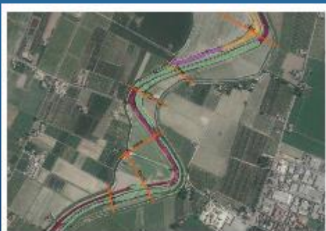
Figure 2. Classification of riparian vegetation: detail of final snapshot with polygons of homogeneous features overlapped to a satellite image. Transversal lines are surveyed river cross sections.
